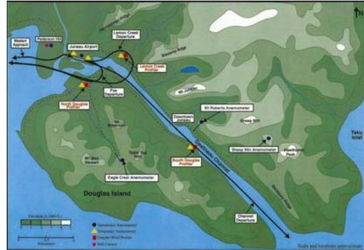
**Figure 2: Map showing locations of anemometers and profilers around the Juneau area.**
