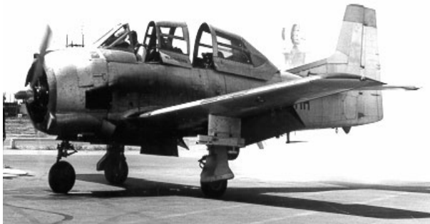
Image circa 1970 showing startup at Rapid City Regional Airport. Note foil impactor under wing.
