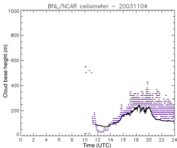
Figure 5. Ceilometer observation of cloud base height (symbols) and the calculated LCL from near-surface data (solid line) at the FAA C&V field site on November 4<sup>th</sup> 2003.
