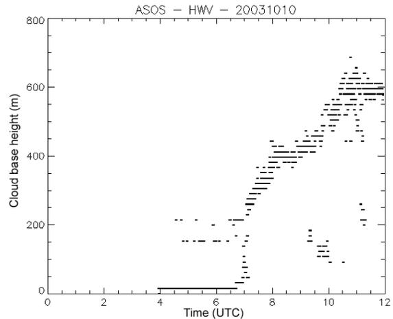
Figure 4. Ceilometer observation of cloud base height at Shirley (HWV) on October 10<sup>th</sup> 2003. Symbols indicate detection of cloud base at every 30 sec.
