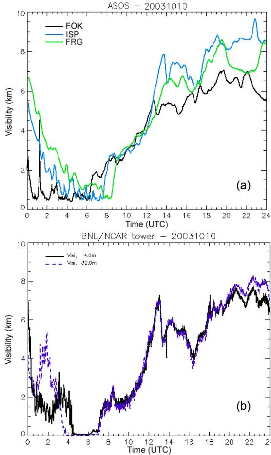
Figure 2. Horizontal visibility observed (a) at three ASOS stations and (b) at two heights (4m, solid line; 32m, dashed line) on the C&V tower, October 10<sup>th</sup> 2003.
