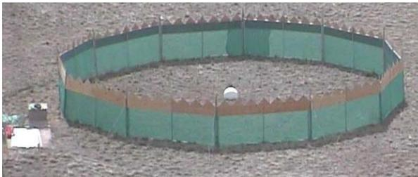
FIG. 3. Photograph of the 50 foot diameter eddy fence. The lower portion covered with a porous green fencing material is 6 feet high.
