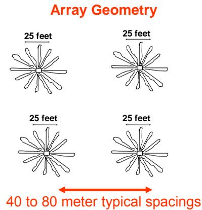
Fig. 4. View of a typical infrasonic observatory array configuration. The exact positioning of the twelve porous irrigation hoses radiating outward from each of the four sensors is not critical.
