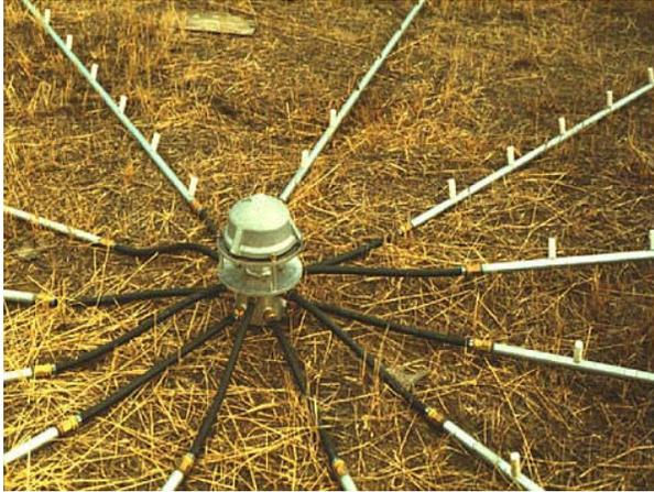
FIG. 2. Photograph of a spatial filter for reducing wind-induced pressure fluctuations in the infrasonic frequency range.
