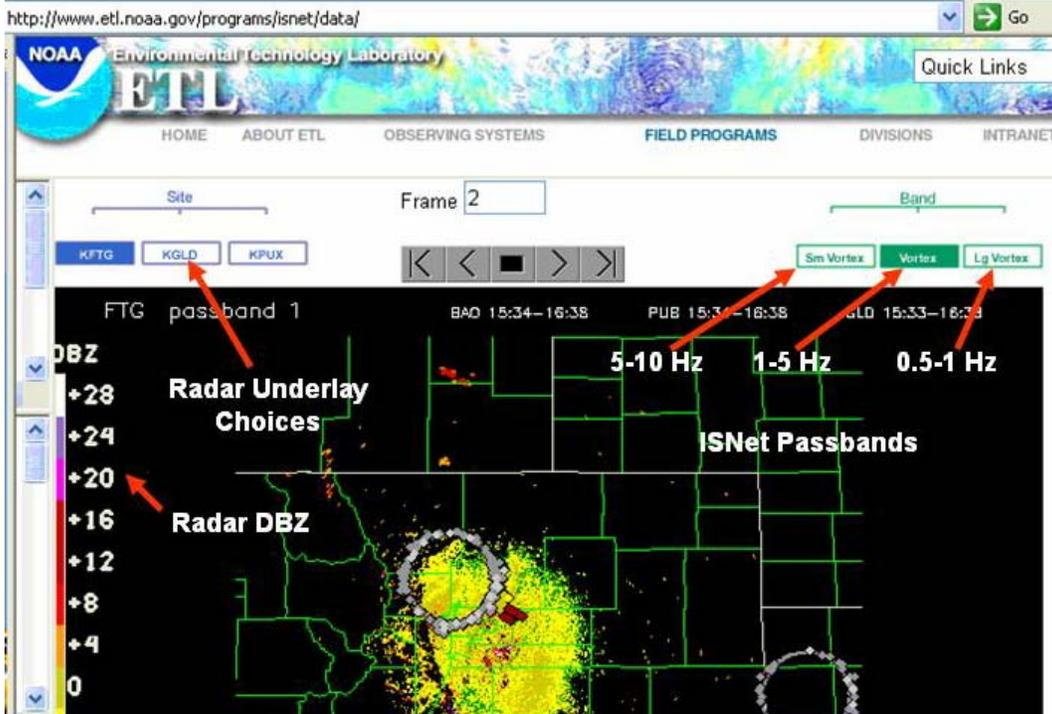
FIG. 20. An example of an actual web display showing the BAO and Goodland ISNet sites. The options for choosing radar underlays and infrasonic passbands are indicated. The 1-5 Hz passband is usually chosen for display. A signal is being detected at the BAO from the SE during this interval.
