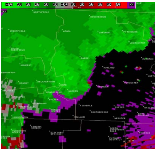
Figure 12. 0.5° Storm Relative Motion image from the Taunton WSR-88D, at 1920 UTC. Note green/red couplet in center of image.
