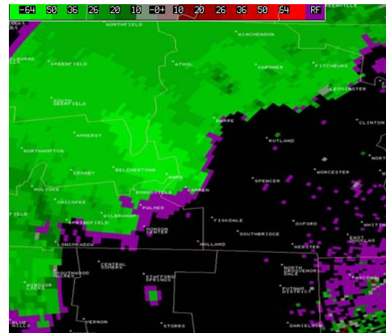
Figure 10. 0.5° Base Velocity image from from The Taunton WSR-88D, at 1915 UTC.
