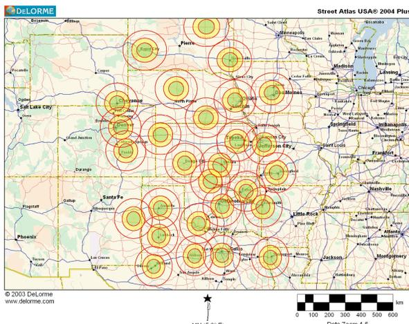
**Fig. 1** The elevation of the 0.5° beam in the WSR-88D network across the plains, showing regions below 0.5 km (green), below 1.0 km (yellow and green), and below 2.0 km (outermost red-rings).
