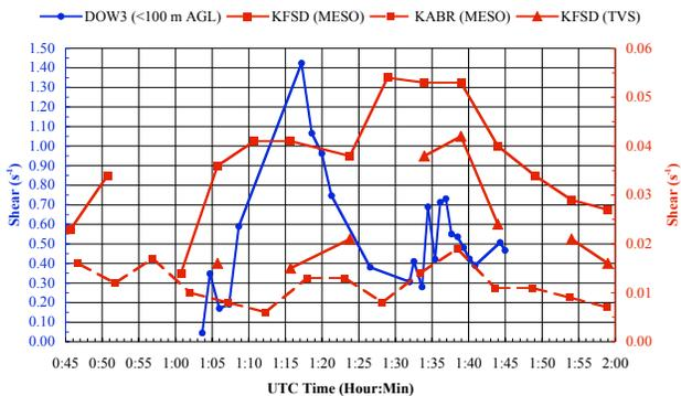
**Fig. 3** The shear across the 30 May 1998 Spencer, SD tornado and supercell mesocyclone as viewed by DOW3 (blue) or the WSR-88D MDA/TVS algorithms (red). The KFSD observations are near and above 1 km AGL, while the KABR observations are near and above 3 km AGL.
