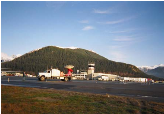
Figure 7: The Univ. of Oklahoma/NCAR Doppler on Wheels mobile scanning X-band weather radar.
