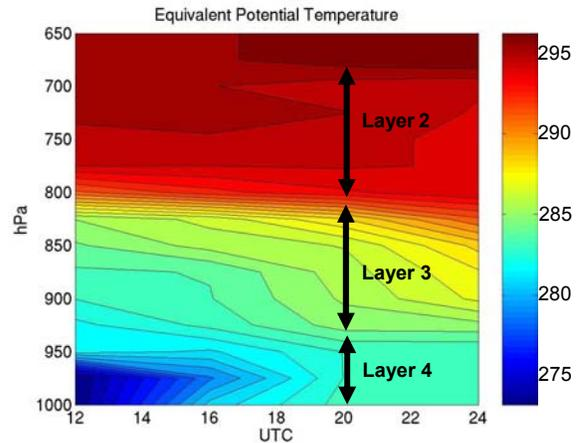
Figure 5. Time series of a vertical cross section of  $\theta_e$  for the lower atmosphere using the KGRB 26/12, 27/00 soundings and the 26/20 aircraft sounding. Layers 2 – 4 are indicated.
