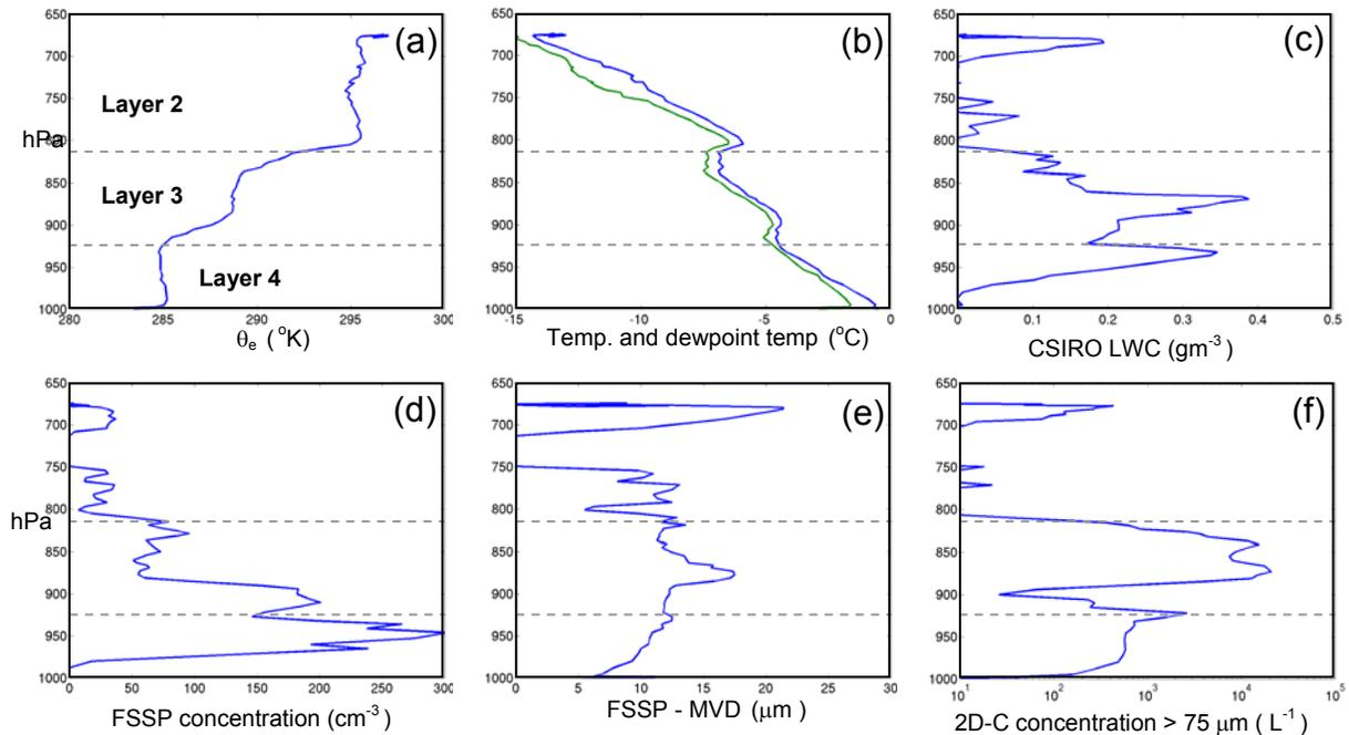
Figure 6. Thermodynamic and microphysical vertical profile of the cloud at KGRB from the Twin Otter. (a) Equivalent Potential Temperature ( $^{\circ}K$ ), (b) Temperature and dewpoint temperature ( $^{\circ}C$ ), (c) Liquid water content ( $gm^{-3}$ ), (d) FSSP-concentration ( $cm^{-3}$ ), (e) FSSP-median volumetric diameter ( $\mu m$ ), (f) concentration of particles larger than  $75 \mu m$  for the 2D-C Gray ( $L^{-1}$ ).
