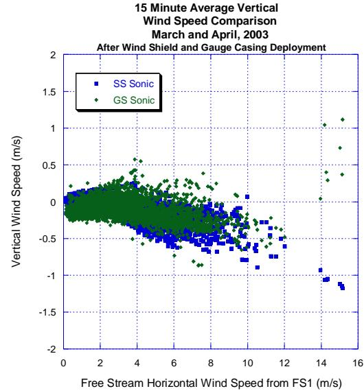
Figure 4 – Comparison of vertical wind speeds inside the shields versus the horizontal free stream wind.
