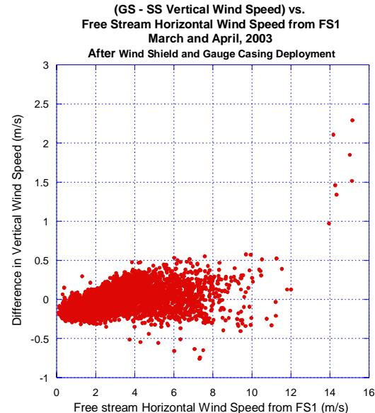
Figure 5 – Difference in vertical wind speed from shielded sonic anemometers versus the free stream horizontal wind.
