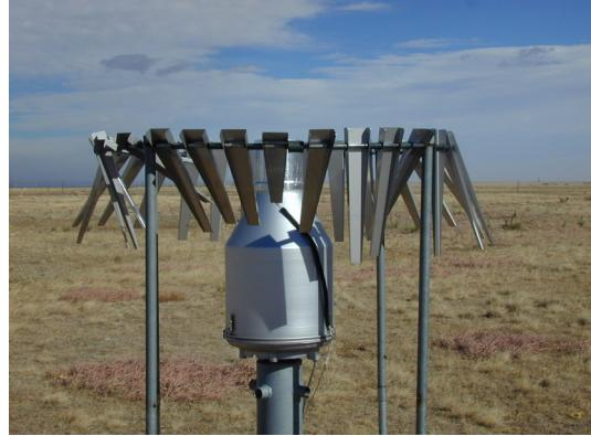
Figure 7 – The deflection of the single Alter slats during a high wind event.
