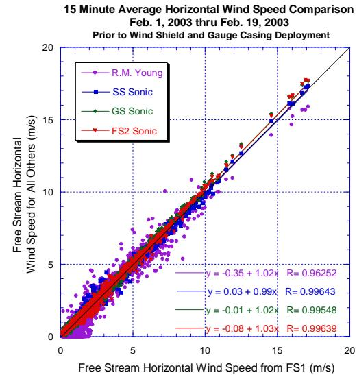
Figure 2 – Comparison of horizontal winds from all sonic anemometers before shields were installed.
