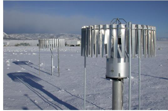
Figure 1 – View of the sonic anemometers inside the single Alter shields. The one in the foreground has the GEONOR casing inside.
