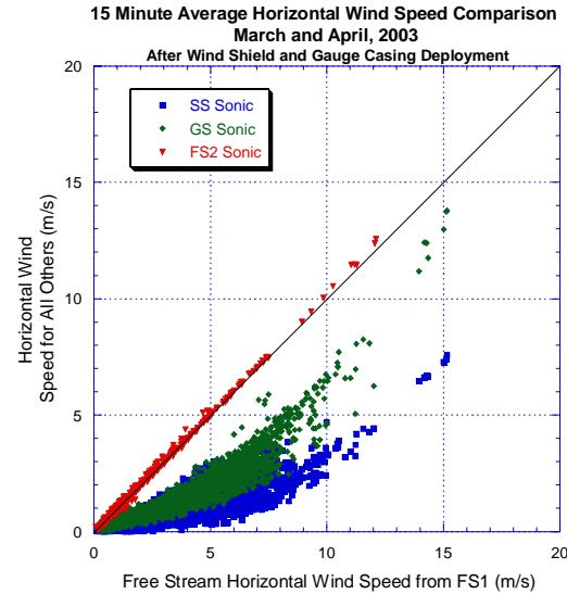
Figure 3 - Comparison of horizontal winds from all sonic anemometers after the wind shields and GEONOR casing were installed.
