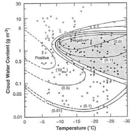
Figures 1a, 1b, 1c: Laboratory results in the diagram of temperature ( $^{\circ}\text{C}$ ) and cloud water content. Included are results from 1a) Pereyra et al (2000) 1b) Takahashi (1978); and,
