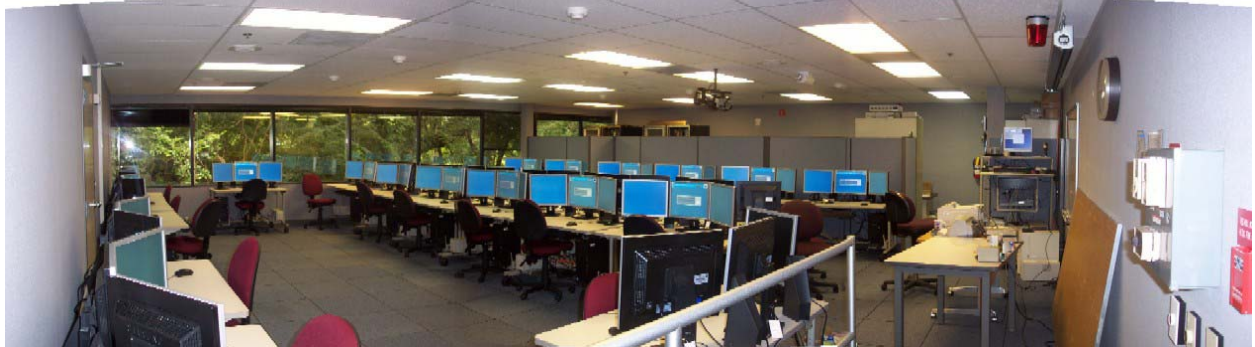
Figure 1: WDTB Research and Training Lab has 25 three-headed networked Linux workstations running Weather Event Simulator (WES) software. (Photo by Ed Mahoney)
