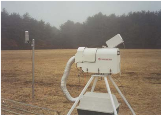
Figure 1 – The Microwave Profiling Radiometer at the Brookhaven National Labs site.
