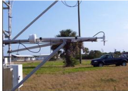
Figure 3. A mechanically aspirated 1.8 m temperature sensor at tower ID#0403.
