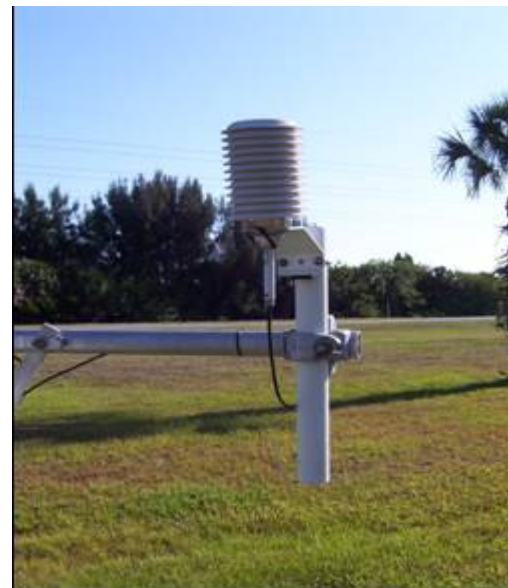
Figure 4. A naturally aspirated 1.8 m temperature sensor with radiation shield at tower ID#1007.
