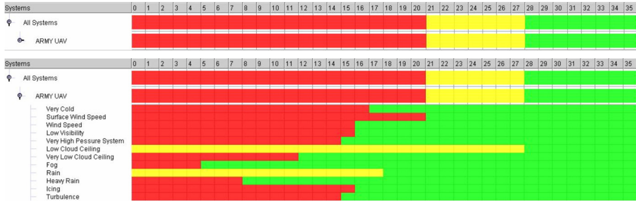
Figure 3: Current IWEDA-like temporal display showing the predicted T-UAV capabilities (top), and the expanded tree view showing the results of the individual rules (bottom) extracted from one particular grid point within the PUMAR domain. The NWP forecasts extended for 36 hours (the intervening hours were persisted for display purposes). The red, yellow and green “pixels” were assigned based on operational T-UAV weather sensitivities.
