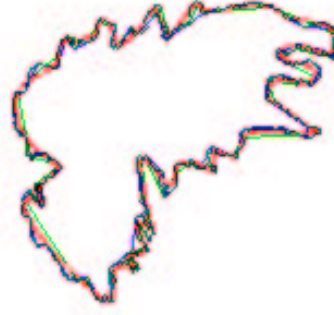
Figure 4: The raw contour of Fig. 3 (black line), and its reconstruction using our scheme (red), the method by Burdon (2003) (green) and the method by Gertz and Grappel (1994) (blue).
