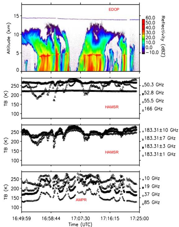
The co-located CAMEX-4 observational data set including EDOP, HAMSr, and AMPR measurements from the NASA ER-2 Aircraft
