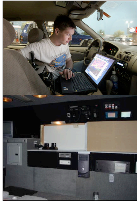
Figure 4: Inside the student-equipped chase vehicle (Top); and the MESO vehicle (Bottom); showing laptop and desktop computers connected with cellular, GPS, and XM MTN technologies giving a sophisticated mobile forecasting capability in the field.
