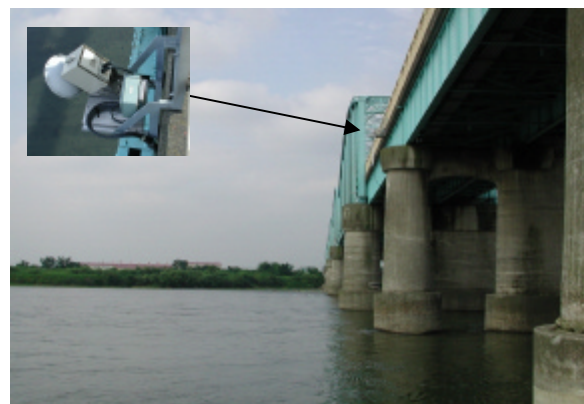
Fig.6: Yattajima observatory of Tone River and RF current sensor.
