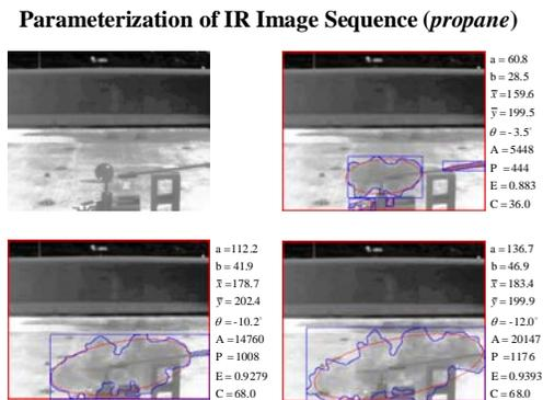
Figure 8. IR images of propane expansion, with complete record of shape parameters
