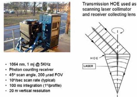
Figure 1. Holographic lidar principle (right) and HARLIE lidar apparatus (left)
