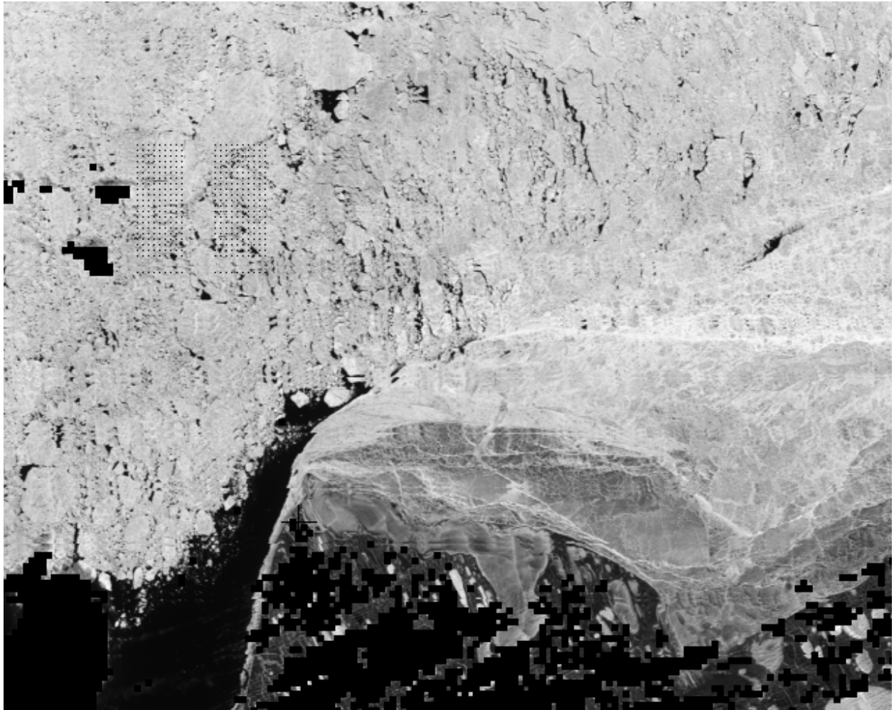
Figure 4: MODIS band 1, 250m resolution, June 13, 2004. Black dots are Aerosonde digital camera image locations (center points), black squares are from the MODIS cloud mask. Barrow is marked by a black +.
