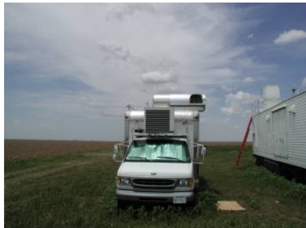
Figure 1 - GLOW Doppler lidar deployed in Oklahoma during IHOP_2002
