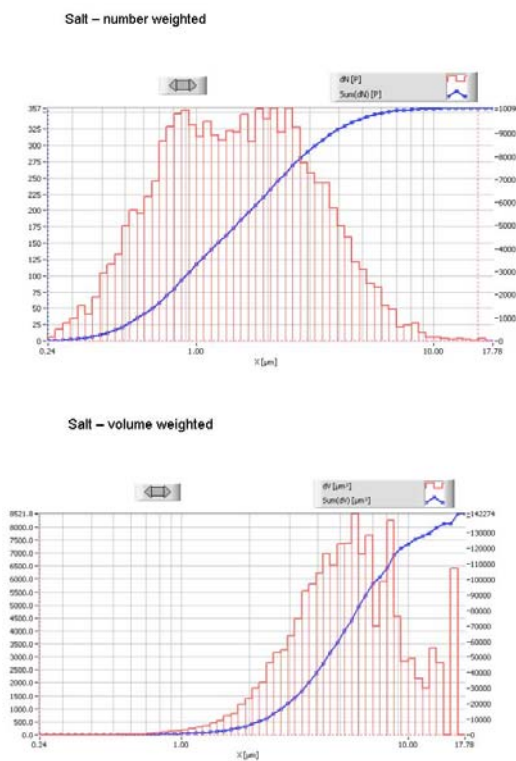
Figure 6: Particle size distribution of the salt powder after it was dispersed from the aircraft. Background concentrations are negligible. The abscissa is the particle diameter, and the left ordinate is the concentration density by numbers on the top panel [dN/d\ln(D)] , and by volume on the bottom panel [dV/d\ln(D)] . The right ordinate provides the negative of the cumulative distribution of the particles.
