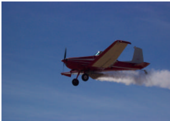
Fig. 2 Photograph of the SOAR salt seeder dispensing processed salt.
