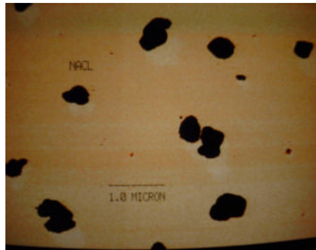
Fig.1 Photograph of processed salt particles viewed with an electron microscope. A size reference is provided in the picture.
