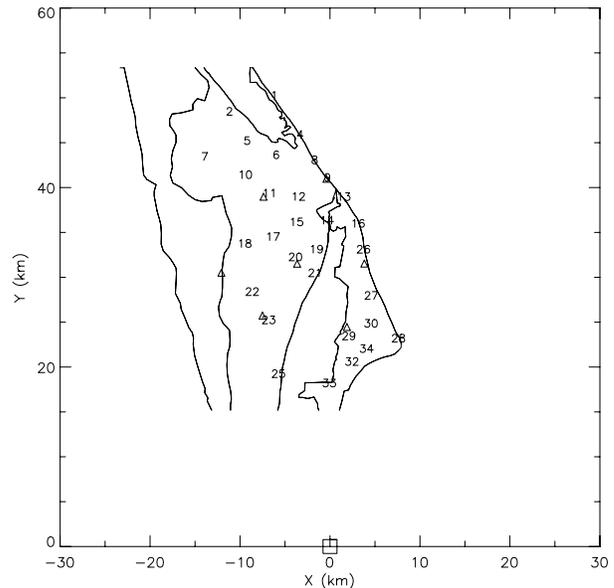
Figure 1: Map of the ground based measurement systems used at NASA-KSC. The WRS-74C is located at the center of the coordinate system and denoted by a square. The electric field mill locations are denoted by their number designation. The LDAR sensor locations are denoted by a small triangle.
