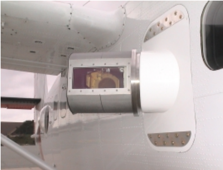
Figure 2 Twin Otter Doppler Wind Lidar (DWL) bi-axis scanner
