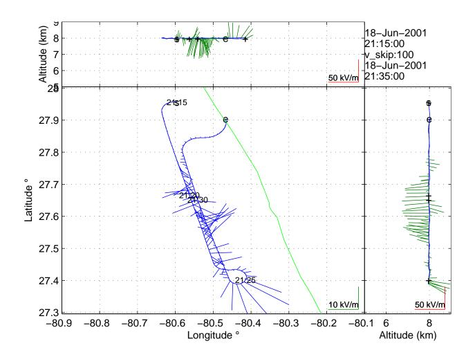
FIG. 2: Plot of aircraft track in *xy*, *yz*, and *xz* and vector electric field in the same plane. Note the scale of the electric field vector are different and are in the lower right-hand corners of each of the three subplots. The start (s) and end (e) of the aircraft track is marked along with minute tick marks.
