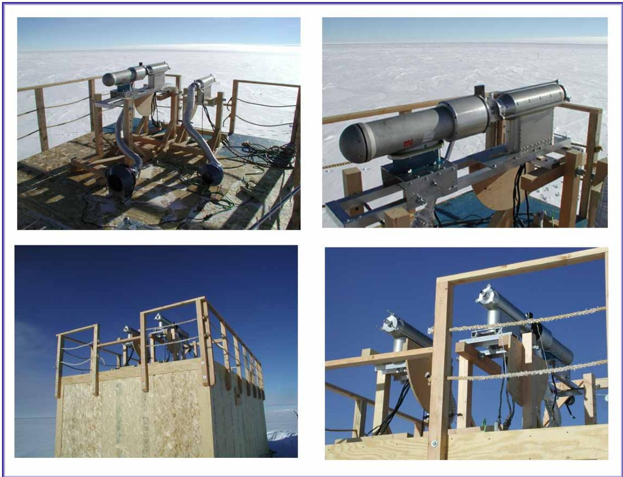
**Figure 1.** Photographs of the SPEC CPIs and LaMP Polar Nephelometer (P-N) on top of a small building at the South Pole. The P-N is seen connected to the exhaust region of the CPI in the panel at the upper left. Both instruments are aspirated using an exhaust fan. The sampling elevation is about 3 m.
