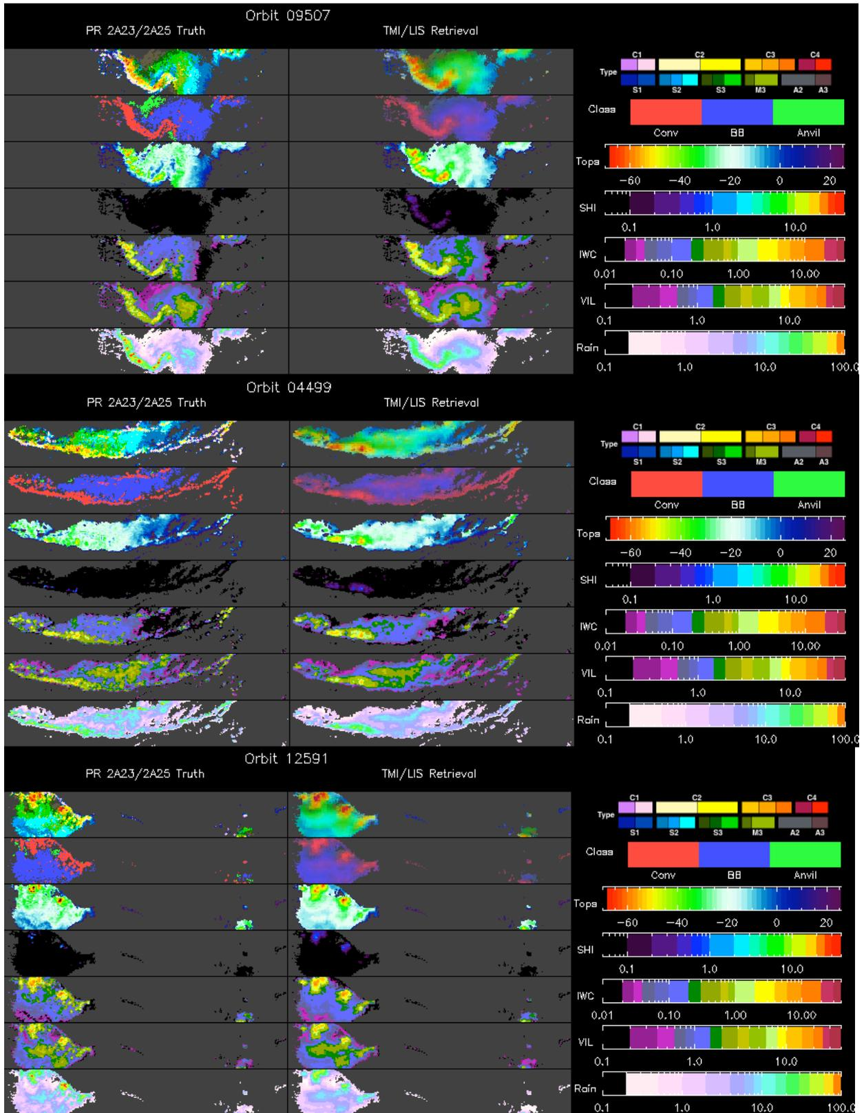
Figure 4 – Sample retrieved orbit swaths (radar truth, left; passive microwave + lightning retrieval, right).
