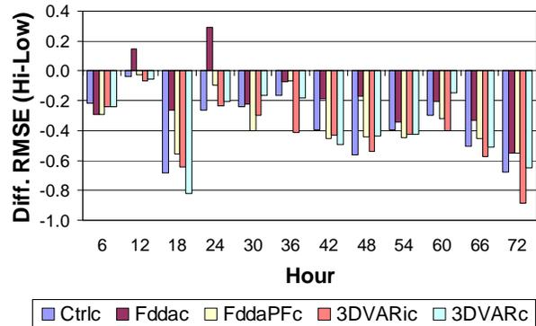
Figure 4 Difference of absolute RMSE for 2-m temperature in experiments Ctrlc, Fddac, FddaPFc, 3DVARic and 3DVARc of high-resolution from those of low-resolution.
