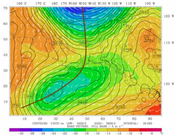
Figure 2 500 hPa geopotential heights (solid black lines), temperature (color shades), horizontal wind vectors (white wind barbs), and trough (thick solid brown line), valid at 12 Z July 26, 2003.
