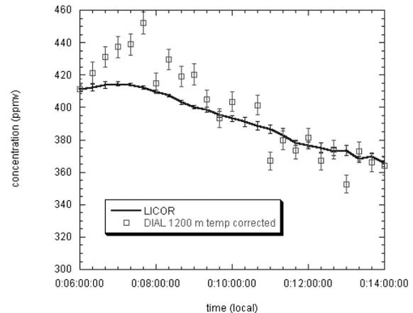
Figure 2: DIAL  $\text{CO}_2$  measurements compared with Li-Cor
