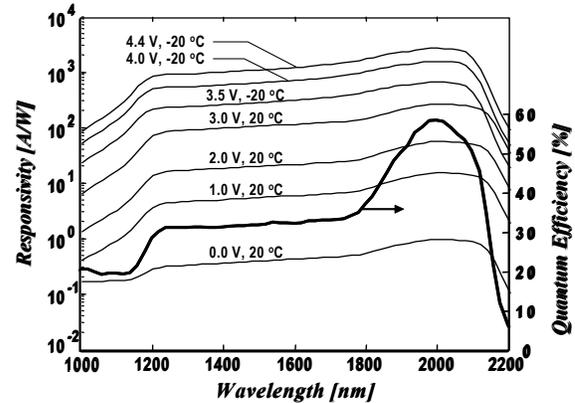
Figure 1: Responsivity and quantum efficiency measurements of AIGAS phototransistor.
