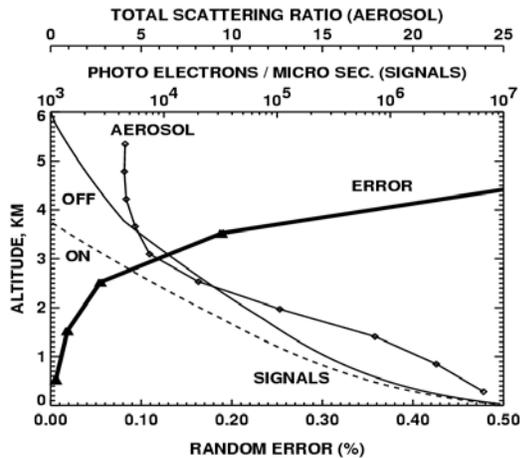
Figure 3: Performance (error) of ground-based DIAL (thick line), on/off lidar signals and assumed aerosol profile are also shown.
