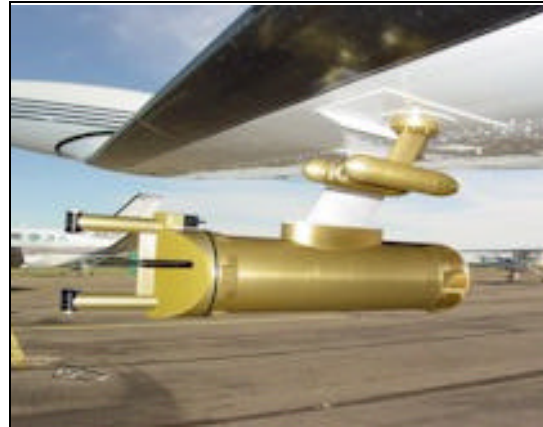
Figure 2b: The DMT CIP probe and the DMT CDP probe.
