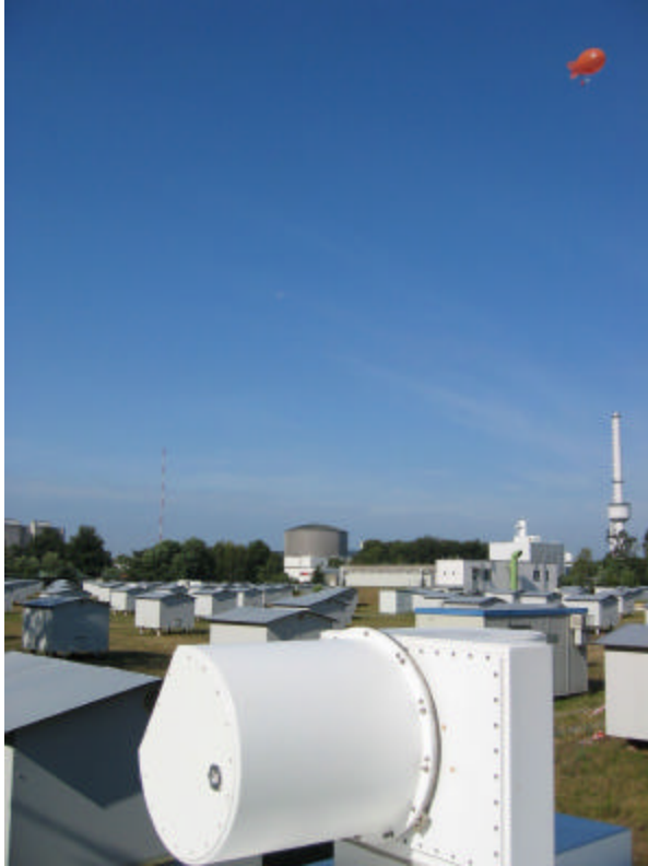
Figure 1, View from the roof of the lidar shelter with meteorological tower (background) and tethered balloon. The white device is the lidar scanner.
