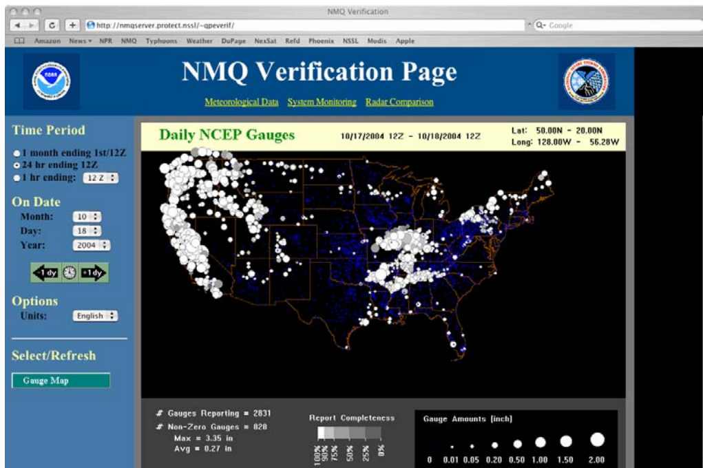
Figure 3. An example display of daily rain gauge observations through the National Mosaic and QPE (NMQ) System/Joint Applications Development Environment (JADE)'s verification web page. The inset shows the scatter plot of radar-only quantitative precipitation estimate (QPE) against the daily gauge observations.
