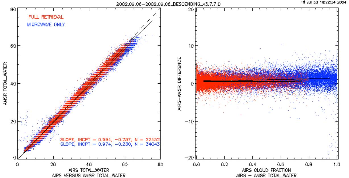
Figure 1. AIRS-AMSR-E comparison for descending (nighttime) orbits on 6 September 2002. Left: Total water from AIRS and AMSR-E for full infrared AIRS retrievals (red) and microwave-only AIRS retrievals (blue). Right: The difference between the measurements as a function of AIRS cloud amount.
