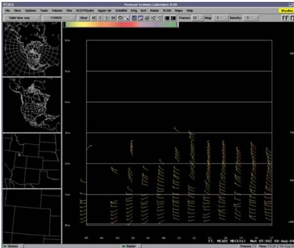
**Figure 5.** AWIPS Cooperating Agency Profiler (CAP) time-height plot for the Ft. Meade profiler provided by the Maryland Department of the Environment. MADIS supports NWS AWIPS users by providing both real-time access to CAP data and instructions for how to ingest and display the data on AWIPS.
