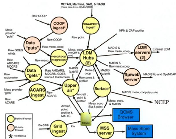
**Figure 7.** A schematic depiction of the MADIS processing environment. FSL is currently in the process of installing "high-availability" pairs for each MADIS processor to help increase the reliability of the MADIS datasets.
