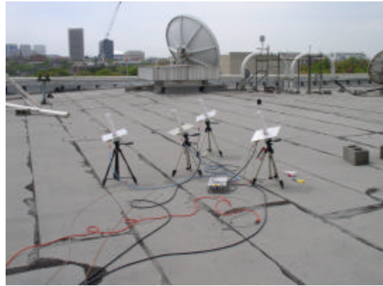
Figure 7 Test setup at Georgia Tech for the S-Band test with 4 element adaptive array used with EO-1
