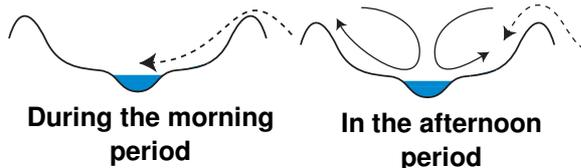
**Figure. 9** Schematic image of the local circulation within the Lake Biwa Basin according to observed data
