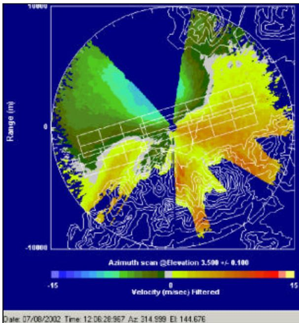
**Figure 6** Sample PPI display of measured radial velocity with an overlay of the airport alerting area and nearby Lantau Island. Flow is out of the NNW.
