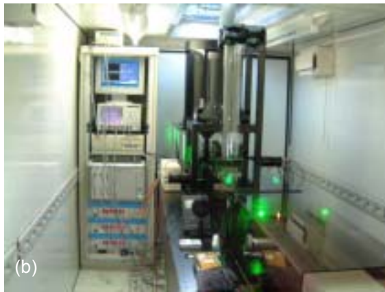
Figure 2: Photographs Illustration and of the lidar system. (a) Aksu Water Balance Experimental Station, Xinjian Institute of Ecology and Geography, CAS. (b) Inside of the lidar container. (c) Illustration of the lidar system.
