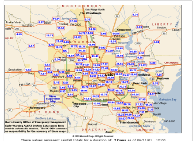
Figure 4. Example rain-gauge network used to bias-correct radar-derived QPEs.
