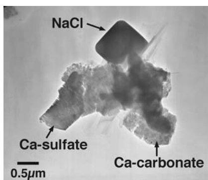
Figure 3: TEM image of sea-salt and partially reacted sea-salt particles over the UAE.
