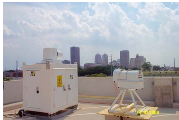
Figure 3. Photograph of the ARL Doppler Wind Tracer Lidar system (left) and the ARL Microwave Radiometer (Measure, etal, 1998) measuring moisture and temperature profiles (right) during the Joint Urban 2003 experiment in Oklahoma City, 2003.
