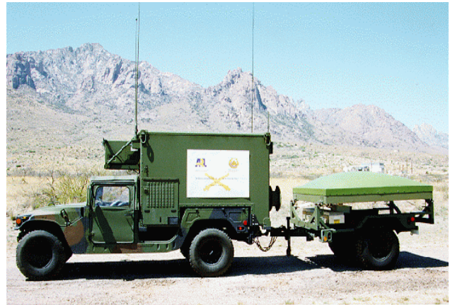
Figure 2. Photograph of the ARL 924 MHz wind profiling radar antenna towed by HMMWV. Processing hardware and software are housed inside the HMMWV's shelter.
