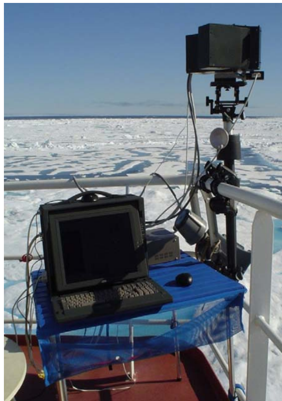
Figure 2. The HEHSI mounted on the forward, portside railing of the Top Bridge of the NGCC Amundsen . The control computer is on the small table, and the camera power supply behind. (The downwards pointing horn beneath the HEHSI is a loudspeaker, and not part of the scientific equipment.)
