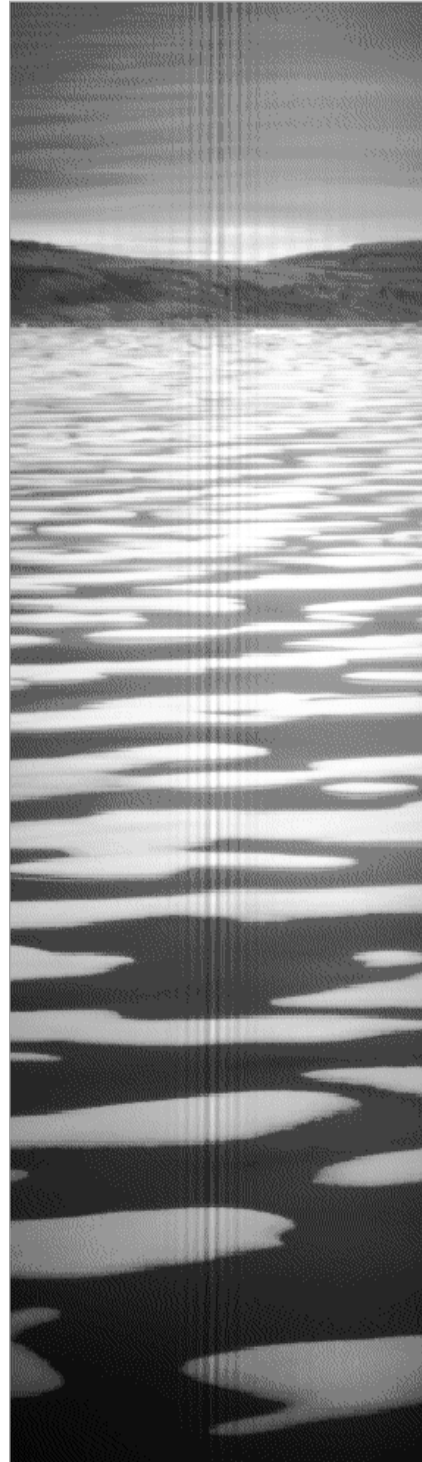
Figure 3. An example of HEHSI data from the ship in land-fast ice at Summer Harbour (70.127°N, 125.081°W) on 15 July 2004. The land in the background is Booth Island to the west of Cape Parry. The interference fringes are the vertical bright and dark vertical modulations of the scene. The frame is 256 pixels wide and 786 pixels high. Each pixel is digitized to 12 bits. The image has been histogram equalized for this figure.
