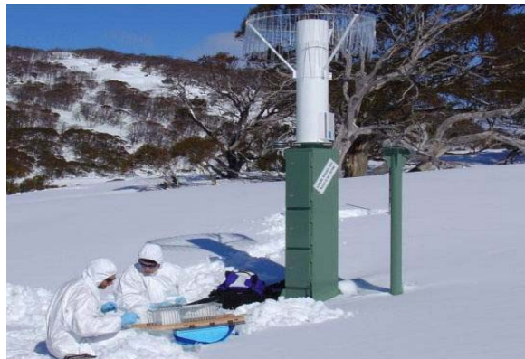
Figure 6. Snow profiling adjacent to a high-resolution precipitation gauge.
