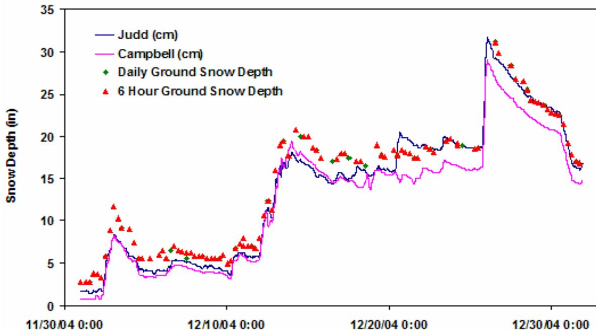
Figure 7: Marquette, MI Total Depth of Snow on the Ground vs. Sensor Depth (in)
