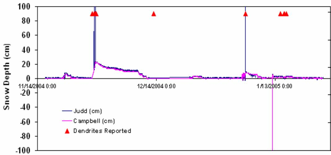
Figure 5: Dendritic Snow Crystals Effect on Sensor Performance Fort Collins, CO.
