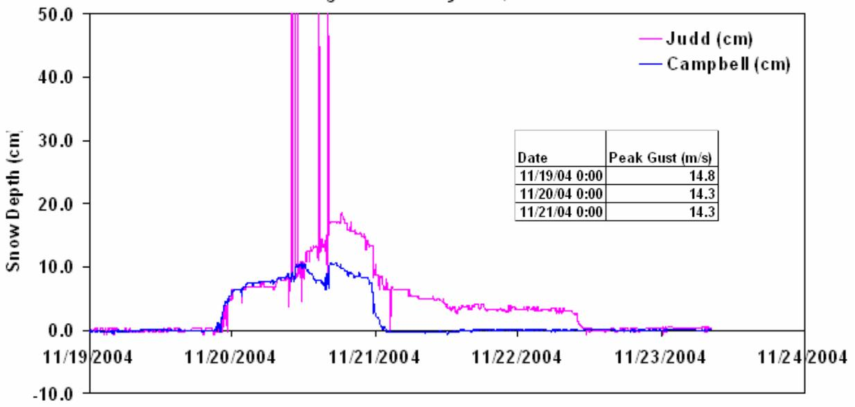
Figure 4: High Wind Effect on Sensor Performance Cheyenne, WY.
