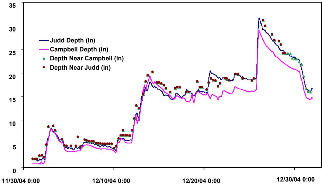
Figure 8: Sensor Depth and Depth of Snow near each Sensor.
