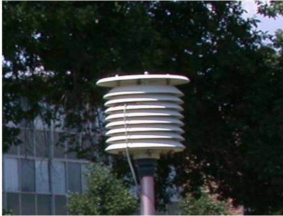
Figure 1. NWS Maximum-Minimum Temperature System (MMTS) radiation shield and display unit.
