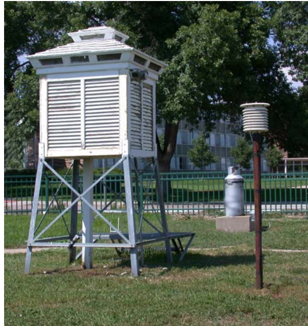
Figure 2. MMTS and LIG thermometer shelters at the Colorado State University campus weather station (05-3005-4) in Fort Collins, Colorado.
