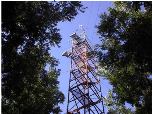
Figure 5. The pecan orchard ET measurement. The Li-Core eddy correlation system is on the top of the 16 m tower.
