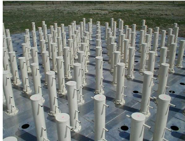
**Illustration 1. Yagi element array on ground plane.**
