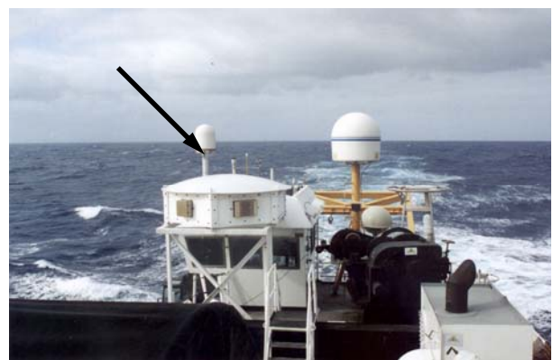
Fig. 1. Electronically stabilized phased-array 915-MHz antenna: R/V Ronald H. Brown (arrow).
