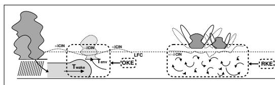
Figure 1. Schematic illustrating the contribution of organized kinetic energy (OKE) and random kinetic energy (RKE) to the cloud-base mass flux in the convection scheme.
